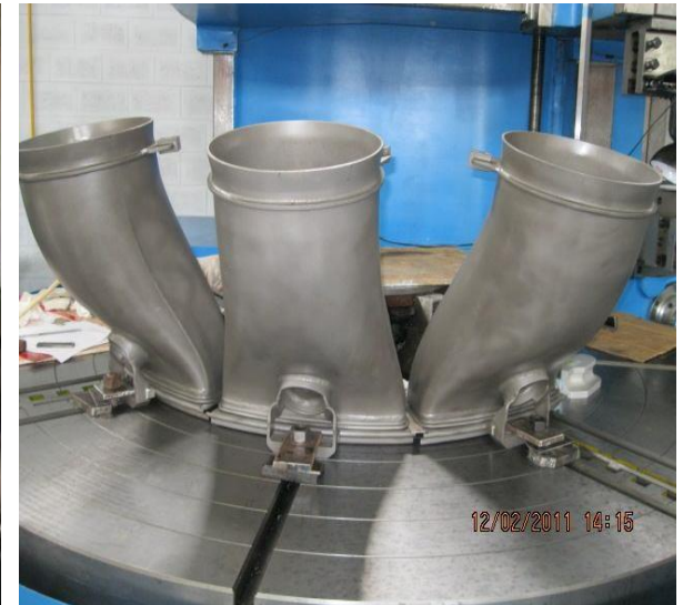
Drop Check on the Vertical of Floating seal Slot Areas
