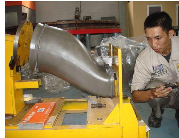
Drop Check on the Vertical of Floating seal Slot Areas
