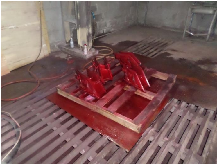
Incoming NDT by Red Dye Penetrant and Mapping finding
