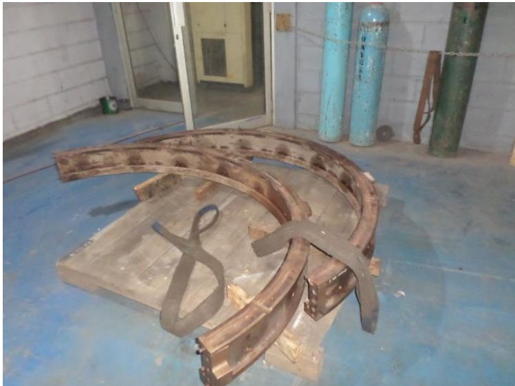
Disassembly Nozzle Segment from Retaining Ring 1st stage Nozzle GE Gas Turbine MS 5002
