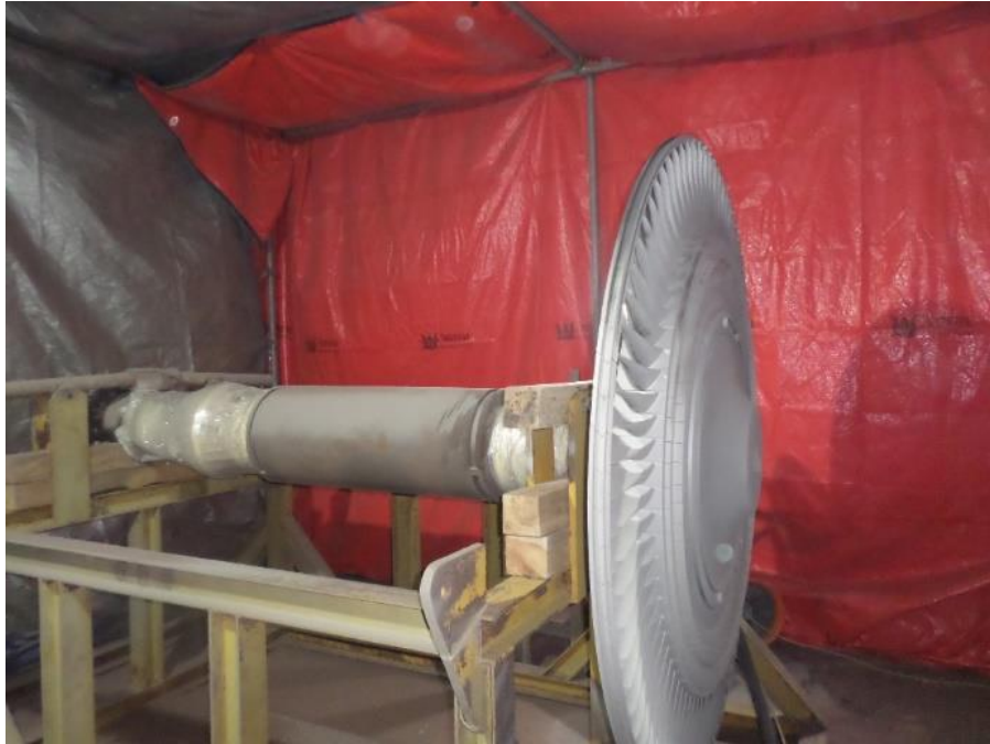
LP Rotor GTG GE MS 5002 after Aluminum Oxide Blast Clean
