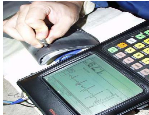
Ultrasonic Test Insures minimum wall thickness requirements are met
