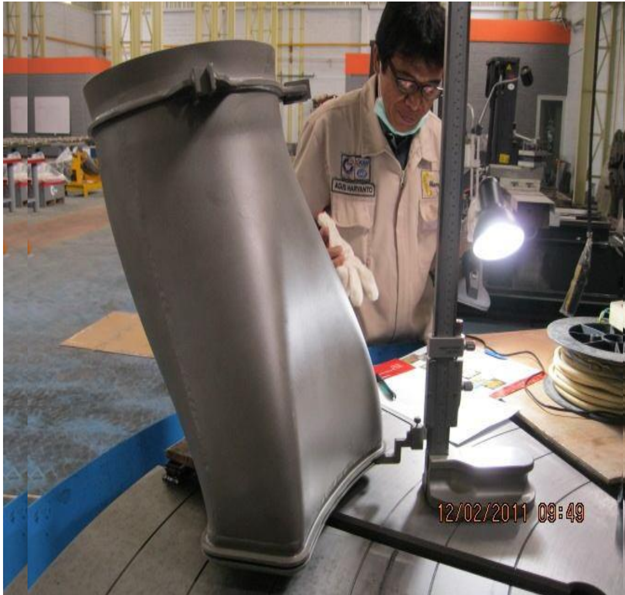
Drop Check on the Vertical of Floating seal Slot Areas
