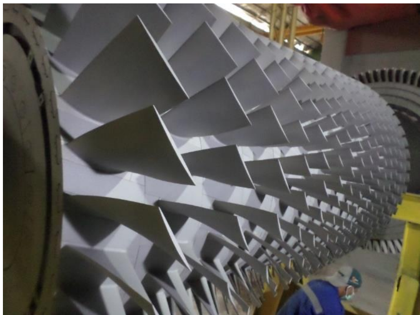
HP Rotor GTG GE MS 5002 after Aluminum Oxide Blast Clean
