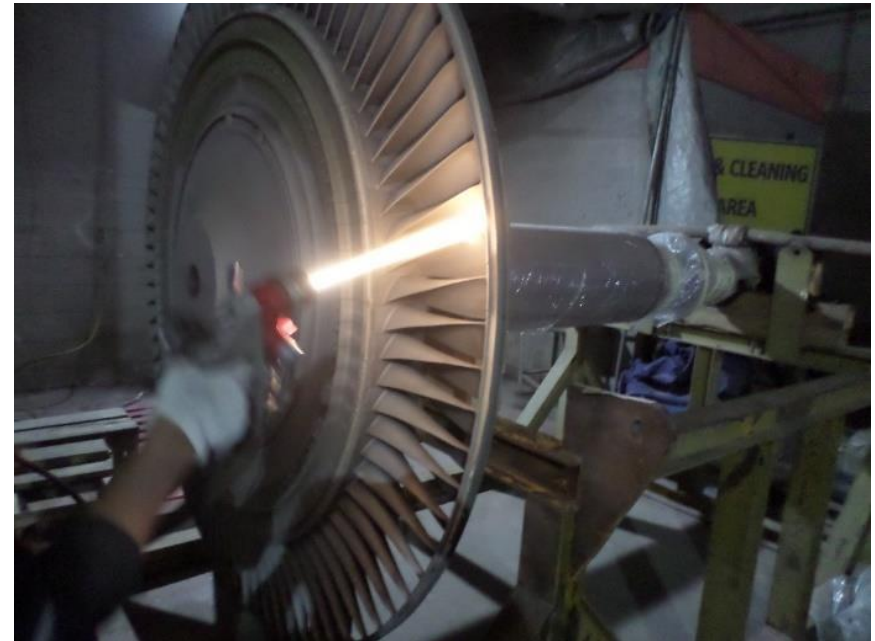
HVOF Coating process on Turbine Blade
