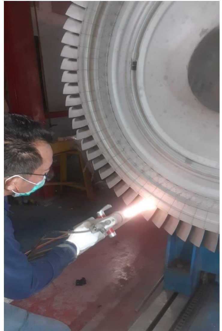
HVOF Coating process on Turbine Blade
