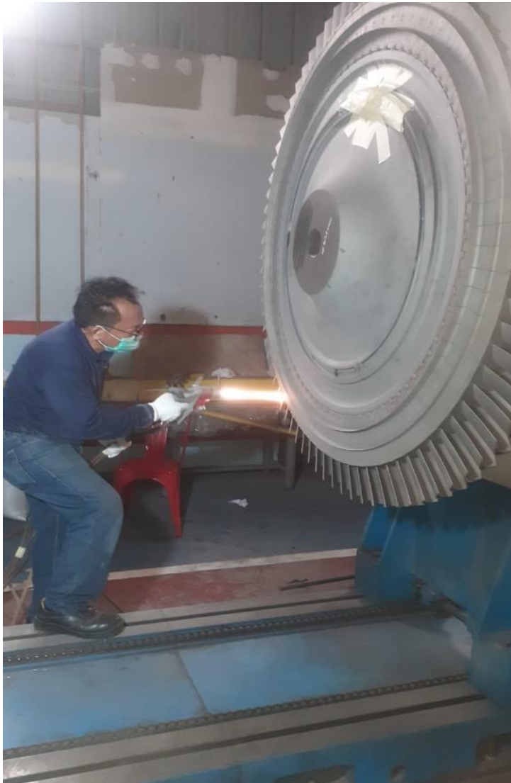
HVOF Coating process on Turbine Blade
