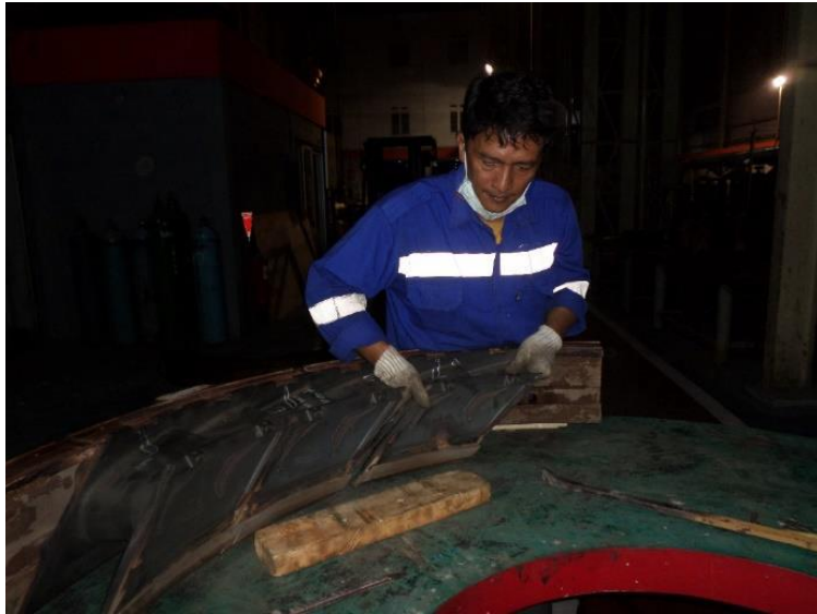
Disassembly Nozzle Segment from Retaining Ring 1st stage Nozzle GE Gas Turbine MS 5002
