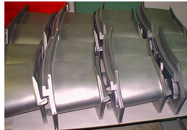
Nozzle segment after Repair
