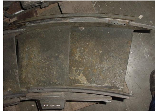
Nozzle segment before Repair
