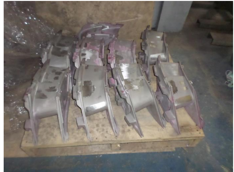
Disassembly Nozzle Segment from Retaining Ring 1st stage Nozzle GE Gas Turbine MS 5002
