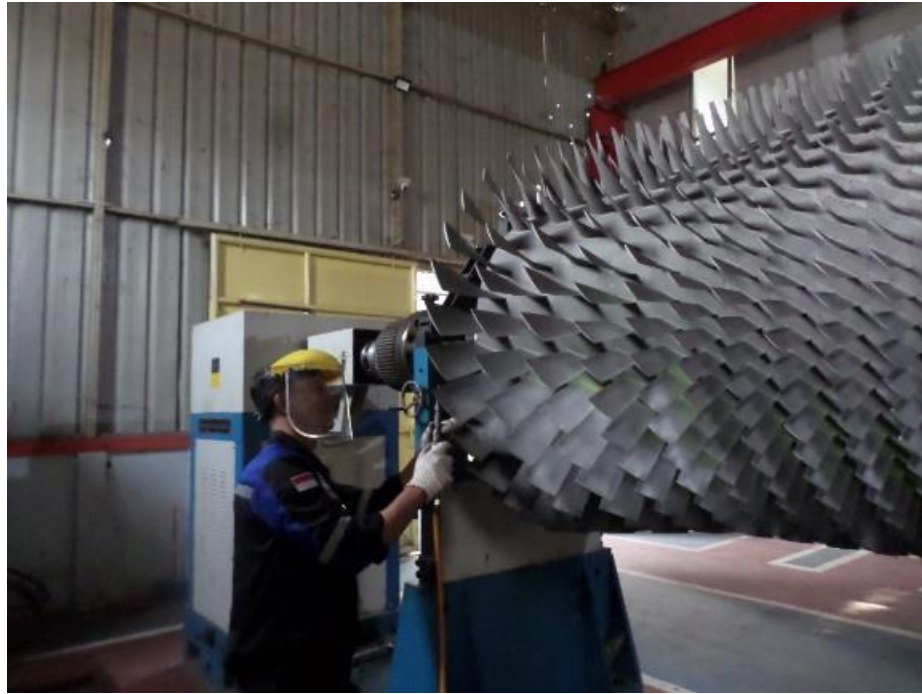
Polishing on Compressor Blade
