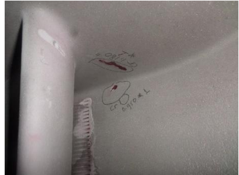
Incoming NDT by Red Dye Penetrant and Mapping finding
