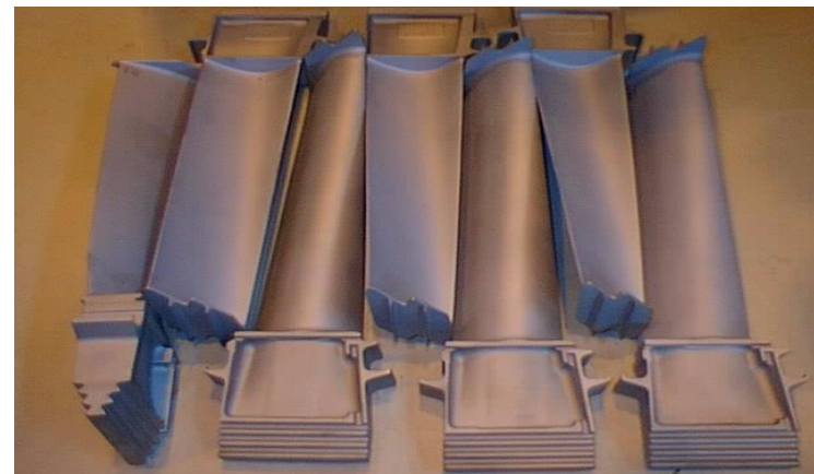
BUCKET AFTER REPAIR
